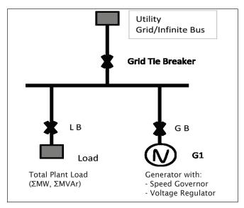
Fig. 3: Generator paralleled with utility grid
