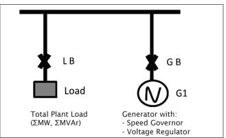
Fig. 1: Stand-alone mode of generator
