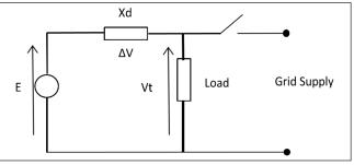
Fig. 6: Equivalent circuit of the synchronous generator operating parallel with the grid
