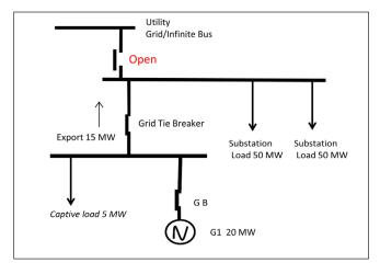
Fig. 5: Loss of grid/utility
