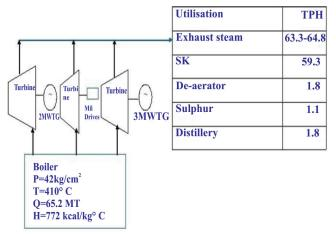
Steam utilization in 3,500 TCD energy-efficient sugar mill
