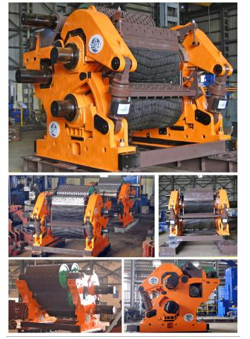
efficiency and performance of the Ulka CMR mills. This is complemented by the fact that, at the same time, power consumption is reduced by about 1.0 kWh per TCH per mill, as compared to the conventional six-roller mill.
